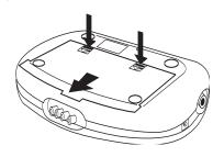
3. Install the batteries as indicated by the polarity symbols (+ and –) marked inside the compartment.
